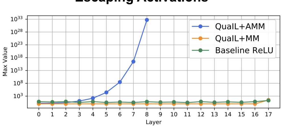
The maximum forward activation values after each nonlinear layer at inference time for using Quail+AMM rapidly increase for deeper networks such as ResNet-18. When using the true minimum and maximum at inference time (QualL+MM), the maximum forward activation values are similar to a baseline ReLU network. Thus a true bounding function is required at test time to guarantee bounds on pre-activation values.
