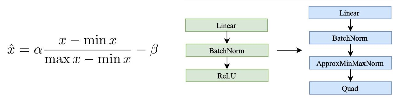
Before each Quad activation, an Approx Min-Max Norm layer is placed in order to bound pre-activation values. This mitigates the escaping activation problem at training time. During training, approximations of both the minimums and maximums are calculated and stored using a weighted moving average of the true minimums and maximums (we use a smoothing factor of 1/10). When performing inference, these stored approximations are then used to perform approximate normalization.
